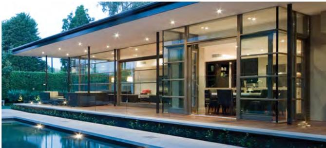
Double or triple glazing together with a double layer of seals and multi-point locking ensure energy savings of up to 84% and a sound protection of up to 45dB. This is some 80-90% over conventional sliding doors.
