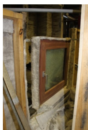
Window after BAL40 preliminary testing, outside, inside
