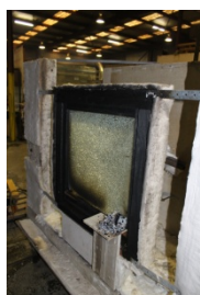
Window after BAL40 preliminary testing, outside, inside
